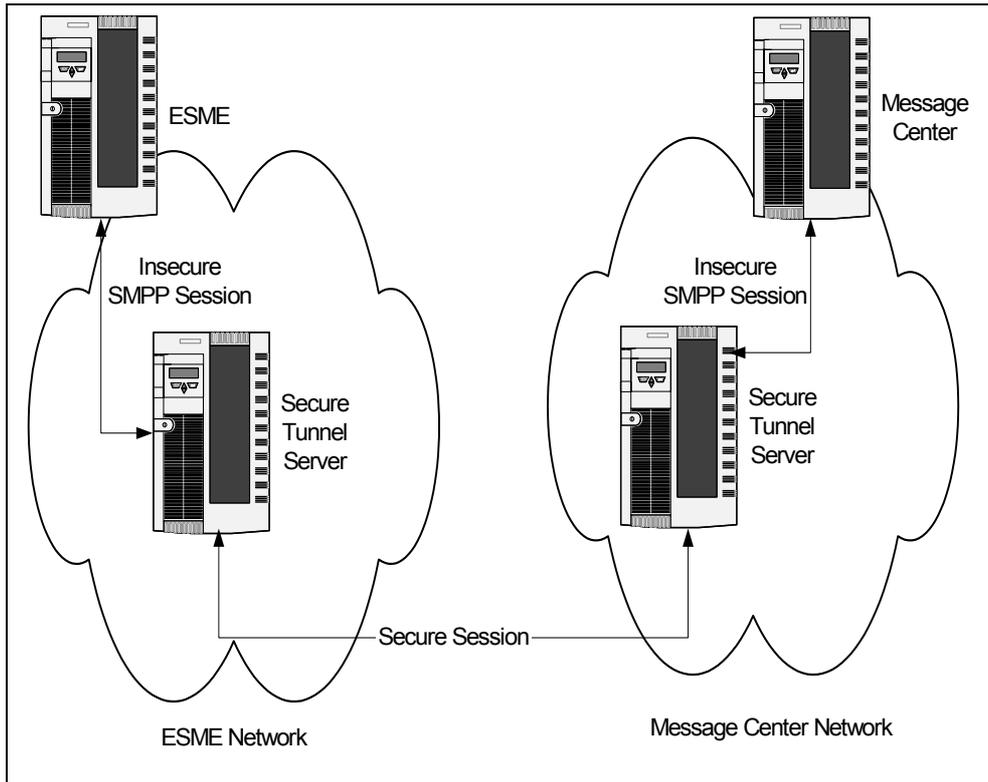
Figure 2-18 ESME-MC SMPP session using a secure tunnel
