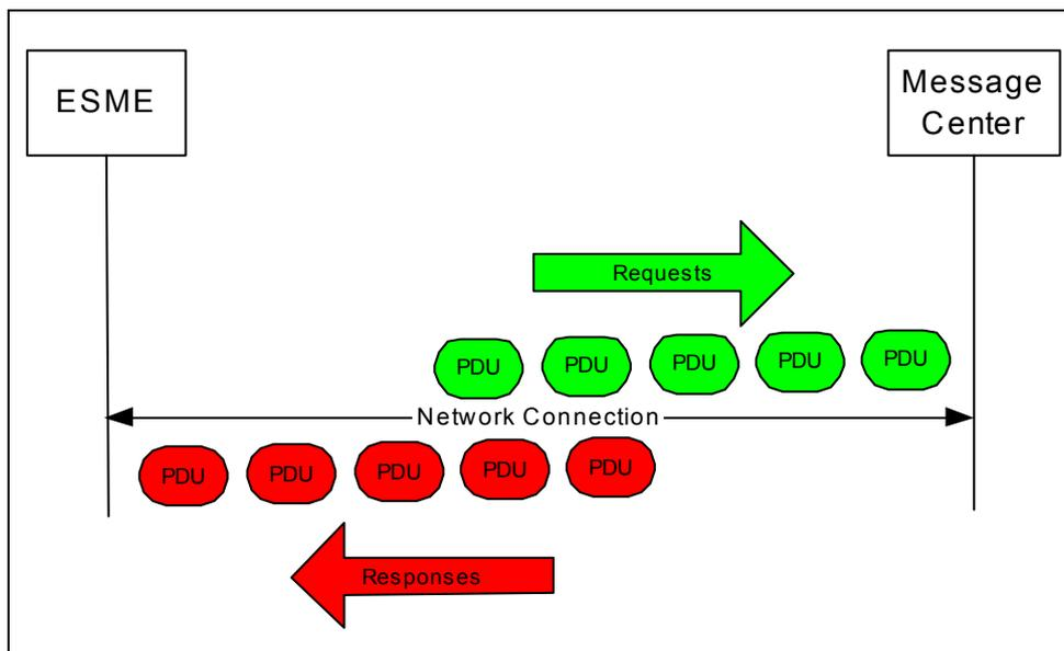
**Figure 2-15 Asynchronous Windowing**
