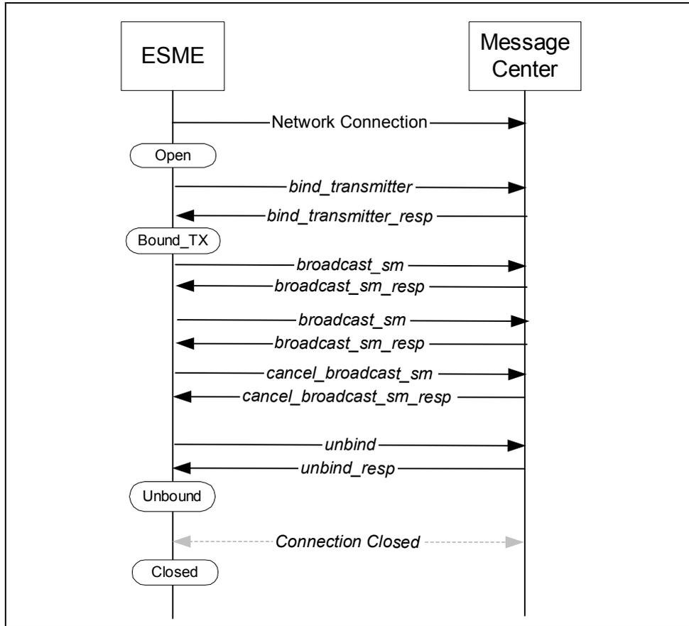
Figure 2-11 Example Transmitter Session (Cell Broadcast Entity)
